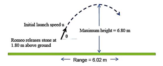
a) Calculate the initial velocity of the stone in terms of magnitude and direction.
