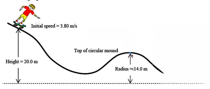
a) Use the principle of conservation of mechanical energy to demonstrate that the speed of the skateboarder at the top of the circular mound is 11.5 m s<sup>-1</sup>.
